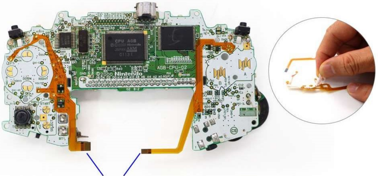
Paste the flex cable on the motherboard
