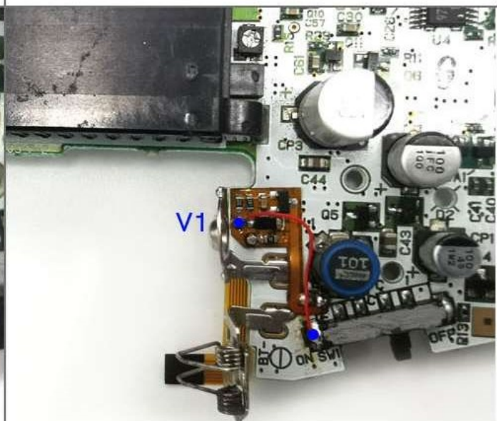
Connect the 'V1' to the ground of the switch.
