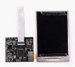
Connect all the flex cable well before power on.
