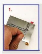
1.Apply the insulating film on the metal surface.
