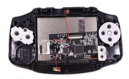
Connect "AV" pad of the black backlight PCB to the "Pin 1" pad of the mainboard of the console by a wire
